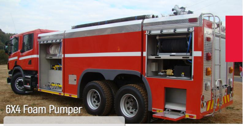
SCANIA P340CB 6X4 CHASSIS, 340HP ENGINE, AUTOMATIC TRANSMISSION, CREW CAB WITH SEATNG FOR FOUR CREW MEMBERS C/W SCBA BACK RESTS
