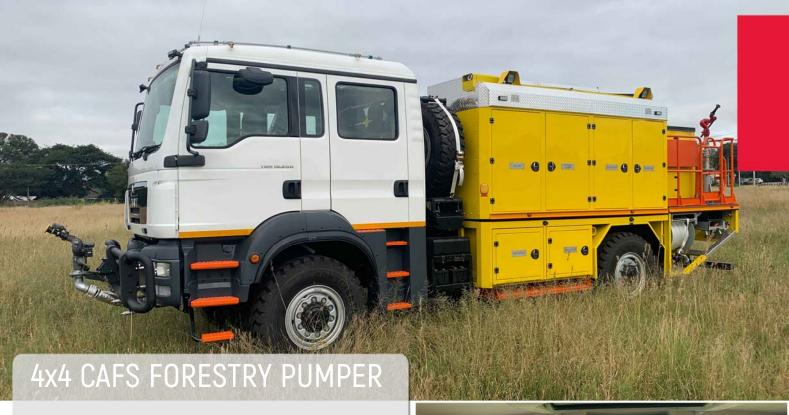
MAN TGM 18.280 4x4 DOUBLE CAB SCBA CREW SEATS IN REAR **RUN FLAT TYRES** SPARE WHEEL LOWERING DEVICE CAB SPRAY PROTECTION **GROUND SPRAY PROTECTION** BUMPER TURRET CONTROLLED VIA JOYSTICK IN CABIN REAR MANUAL CAFS MONITOR DARLEY 3700 L/MIN SINGLE STAGE PUMP WITH 220 CFM CAFS SYSTEM SECONDARY BACKUP PUMP MARCÉ INTEGRATED PUMP CONTROL SYSTEM LARGE STORAGE LOCKERS FIRE BARRIER CURTAINS INSIDE CAB 3000 LITRE WATER 300 LITRE FOAM 500 LITRE RESERVE WATER TANK **FULLY EQUIPPED**
